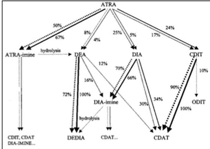
Reaction pathways for molecular ozone and hydroxyl radical reactions are shown with percentages representing relative importance of the pathway. Solid lines represent molecular ozone reactions and dashed lines represent OH radical reactions.<sup>2</sup>
